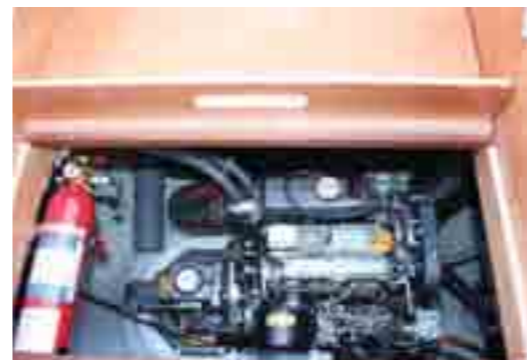
above from left: Hull access to the service points of the 21hp saildrives is available once the marine ply locker base is removed. Photo Kevin Green Swim access is fairly basic with portside ladder but adequate on the Lagoon 39. Photo Kevin Green The cutter rig is ideal for all cruising conditions while the exposed anchor arrangement is simply laid out. Photo Kevin Green below: Essential on all cats, the escape hatches on the Lagoon are breakable in an emergency. Photo Kevin Green
