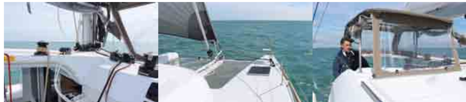
above from left: Mast halyards are nicely near the winches and all other helm sail controls. Photo Kevin Green
